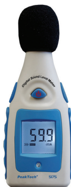
Figure 2. Peaktech Sonometer 5175 (orig.).
